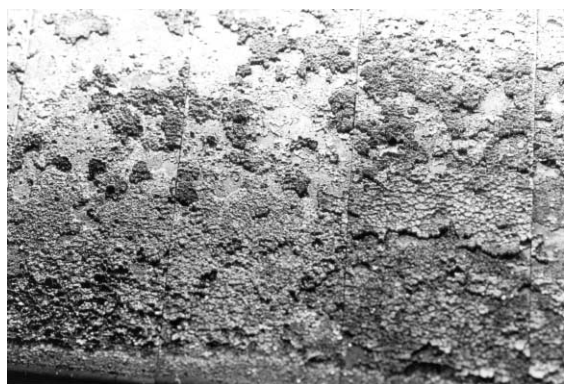
Fig. 4. Neutralizer plate of the ALT-II pumped limiter after 3 years of operation. Blade 8, February 2000. Original size: about 10 \times 15 \text{ cm}^2 .
